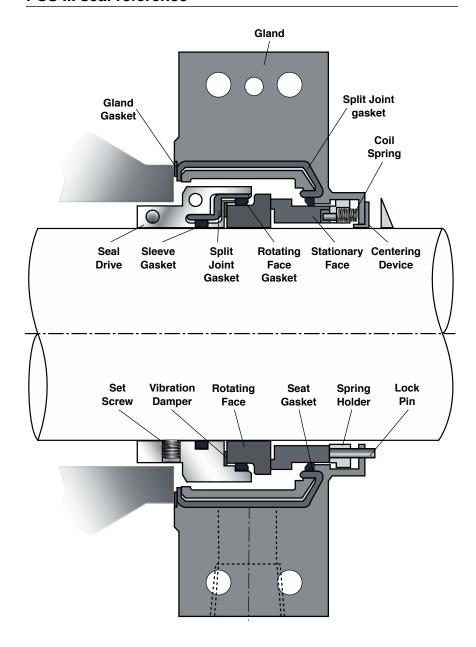
These instructions are to be used in conjunction with the PSS III Repair Kit. The Repair Kit contains replacement seal faces, secondary seals, Loctite <sup>® 1</sup> 430 adhesive, and Dow Corning <sup>® 2</sup> 111 Silicone grease. Other small parts are shown in Figure 1. The repair should be done in a clean, well lit area. The tools you will need to do the repair include:
