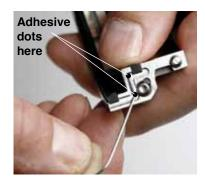
5.4 Put one dot of adhesive near the inner corner.
