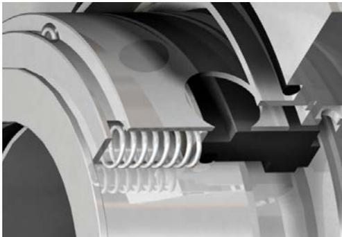
Rotating spring holder with radial openings at both ends of the springs uses centrifugal force to create circulation through the springs. This feature keeps springs clean and properly functioning to accommodate for shaft axial movement and thermal growth.
