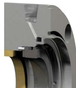
A distribution ring connected to the seal's flush port and located co-axially with the sealing interface improves the cooling efficiency of Piping Plan 11, 14, 21, 31, and 32 by injecting the flush flow 360° around the seal faces.
