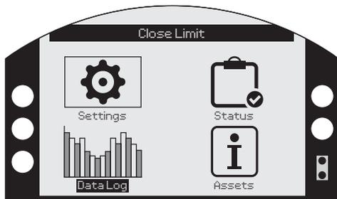
The data can be viewed locally on the dot matrix display and can display pressure and position graphs through to statistical operational data. All data held is secure and can be downloaded using the Rotork *Bluetooth*® setting tool for viewing on a PC with Rotork Insight2 software.
