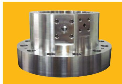
*First-stage seal housing with integral flanges.*
