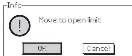
Move the actuator and valve to the Open position and press **⏻** key to select OK. This will set the Open limit at the current valve/actuator position and if not previously illuminated, the Open limit indication LED (factory default red) will be illuminated.
