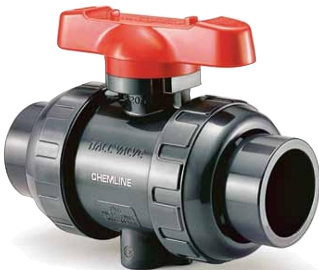
The Chemline Type 21 True Union Ball valve incorporates state of the art features for long term performance. This is a full port, full blocking True Union valve pressure rated at 16 bar (230 psi)<sup>3</sup>. Double stem o-rings and Safety Shear stem design provide for a high degree of safety on hazardous fluid applications. All sizes have an ISO standard actuator mounting platform integral to the valve body. This provides for sturdy and secure mounting of pneumatic or electric actuators.
