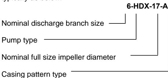
The typical nomenclature above is the general guide to the HDX description. Identify the actual pump size and serial number from the pump nameplate. Check that this agrees with the applicable certification provided.
