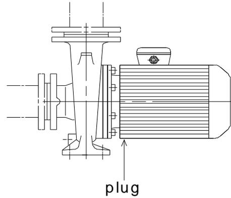
**Fig. 1 Evacuation of condensation water**
