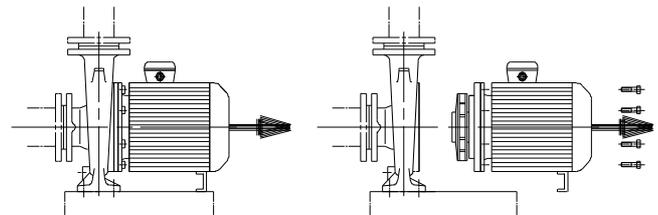
It is possible to disassemble the motor and rotor unit from the pump casing without disconnecting the casing from the piping.
