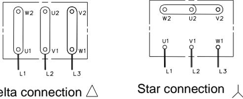
Wire up the motor terminals according to the voltage supply, in accordance with the nameplate fixed on the motor and the connection wiring diagram displayed inside the terminal box, as shown above.
