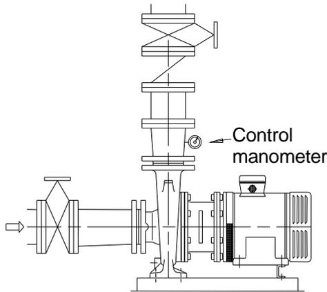
**Installation of control manometer**
