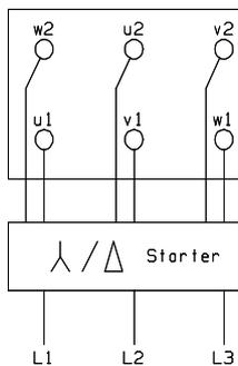
Motors of 3.0 kW or larger may be wired up for star/delta ( $\Delta / \lambda$ ) starting on 380/415 V supply. All connections strips must be removed from the terminal box and 6 wires connected to the  $\Delta / \lambda$  starter, as shown above.
