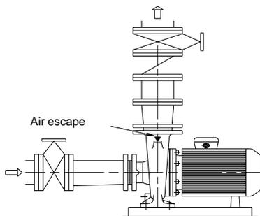
**Priming of a flooded pump**
