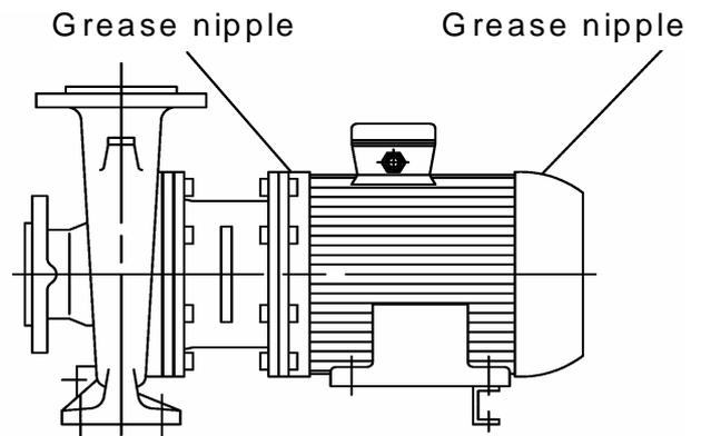
**Fig. 2 Bearing lubrication**
