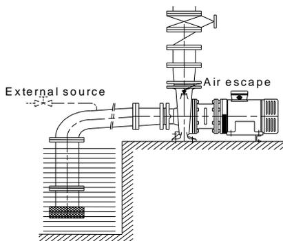
**Priming of sump suction pump with foot valve**
