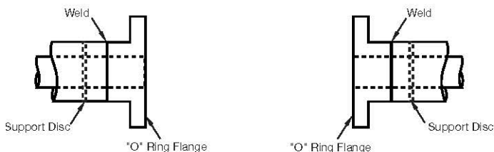
Figure I: Install double-wall flanges
