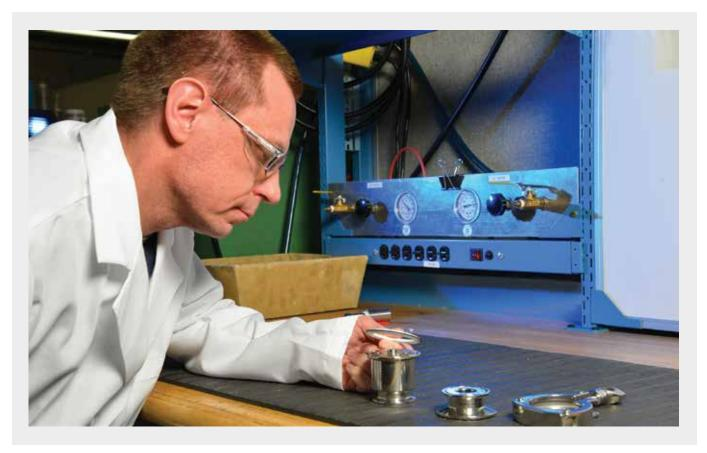
Biopharmaceutical process design and maintenance engineers know that the two most important criteria for choosing a clean steam trap for draining SIP condensate are low subcooling operating and maintenance reliability. Without either, you will have unexpected downtime caused by slow SIP heat-up or validation temperature sensor alarms.
