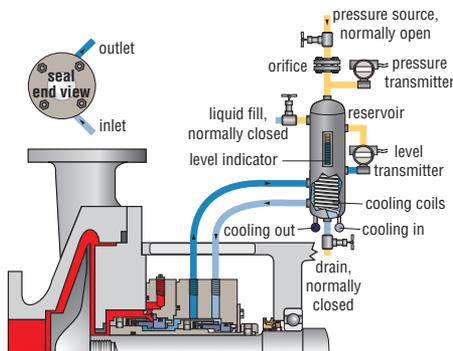
**Plan 54 - Dual seal circulation from an external source** Figure 9
