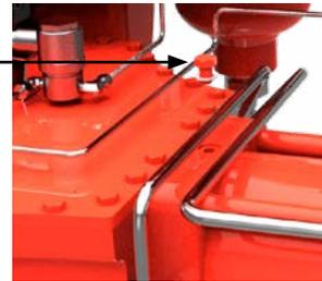
13. Pump (1P1) until oil, free of air bubbles, runs out of hole (R7).
