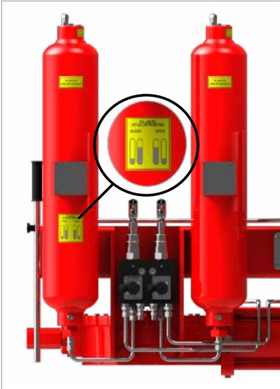
Fig 4.6 Example of Label Oil Level Application
