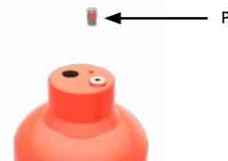
24. Reinstall fitting (N) on gas/oil tanks.
