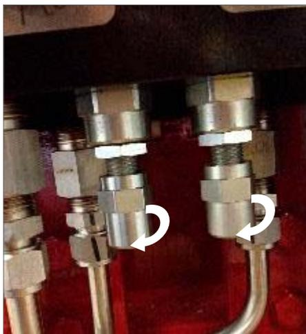
Fig 12.6 Flow regulator cap removal
