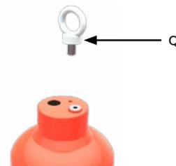
23. Assemble protection plugs (P) into the threaded lifting points of the tanks.
