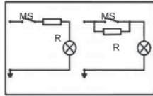
Fig. 2: Lamp load provided with resistance in parallel or series connection to switch of contacts
