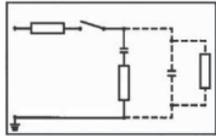
Fig. 1: Protection in case of capacitive loads
