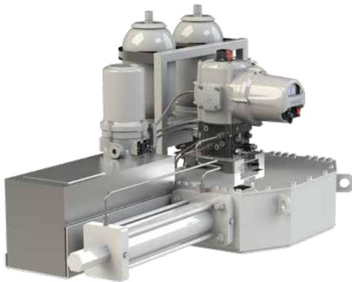
The Skilmatic SI4 quarter-turn actuators offer the flexibility of customisation to suit specific applications and process conditions. The high pressure actuators are self-contained and can operate either a spring-return or double-acting scotch yoke drive. This eliminates the high installation and maintenance costs associated with conventional electro-hydraulic systems which utilise central hydraulic power units.
