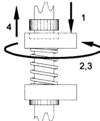
**NOTE:** Factory setting is top switch = CW (closed), second switch = CCW (open), third switch = CW, and fourth switch = CCW.
