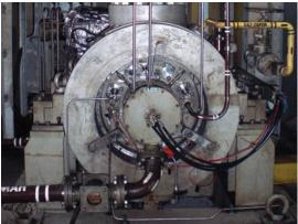
Upgrading a fertilizer plant's hydrogen recycling operation from wet seals to Gaspac dry gas seals took just 19 weeks, and assembly and start-up of the retrofitted machine took just seven days.
