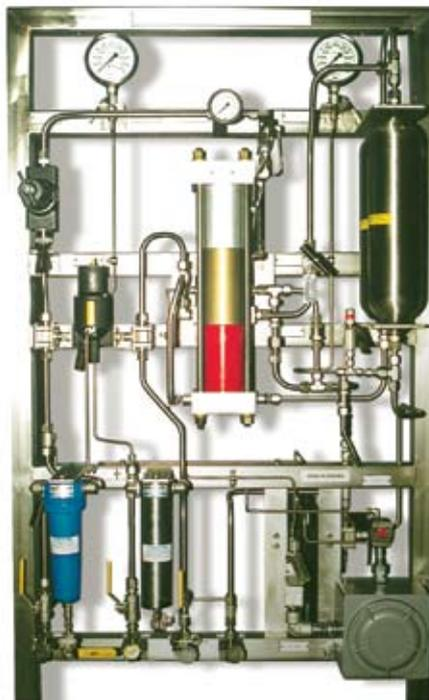
Flowserve **Cleanpac** gas conditioning system eliminates those contamination issues by removing particulates as fine as 0.3 micron and as much as 10% by volume of liquid slugs.
