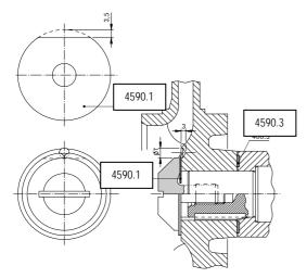
Figure: Locking impeller screw
