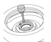
Figure : Removing the case
