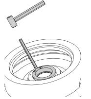
Drill two holes along the centre line of the upright edge of the case wearing ring, see Figure. Drill both holes not deeper than the measured height of the case wearing ring.
