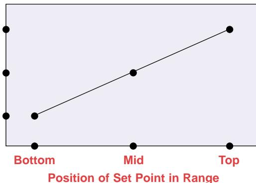
Temperature switch deadbands are a result of the characteristics of the vapor pressure curve as well as other factors. Normally, this results in a deadband which is narrower in the top third of the range than in the bottom third of the range. The values published are nominal and representative of mid-range set points.
